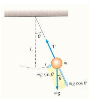
A simple pendulum consists of a mass called a bob, which is attached to a fixed string.
