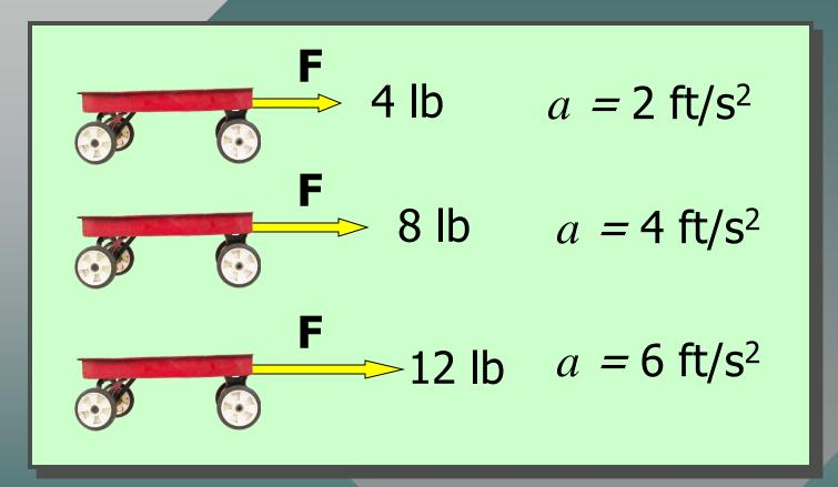
Acceleration a is directly proportional to force F and is in the direction of the force. Friction forces are ignored in this experiment.
